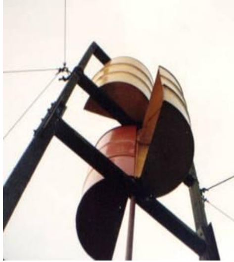
Figure 13: VAWT (Savonius type) for electricity generation
